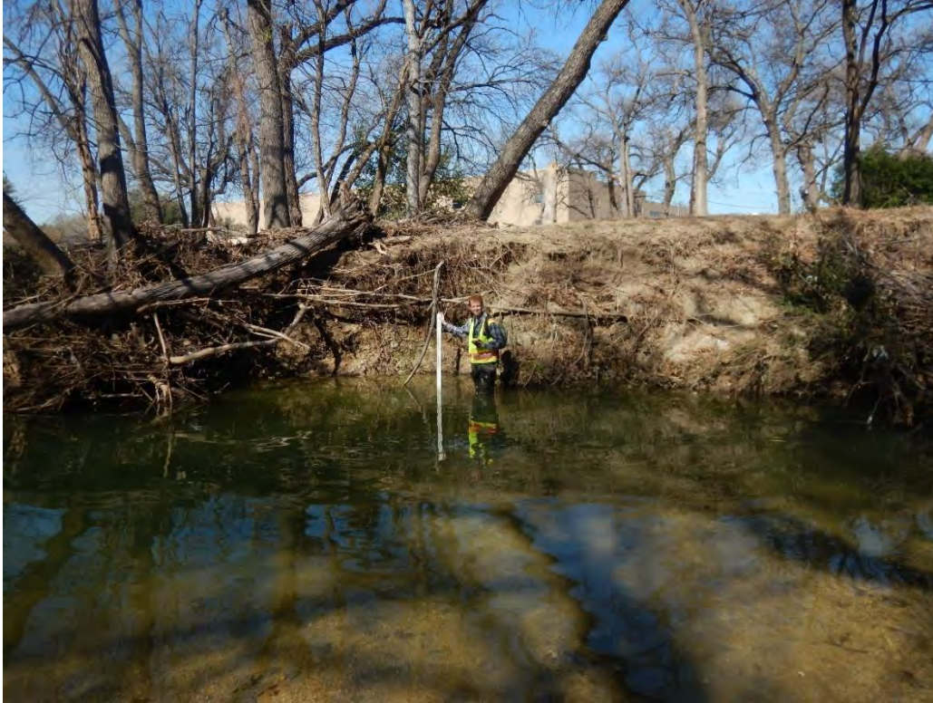
Photo 41. These vertical right banks with leaning trees and slumps have high erosion potential (photo taken looking at the right bank).
