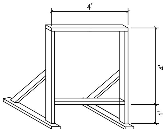
SIGN PANEL 3/4" EXTERIOR PLYWOOD PAINT AS SHOWN ON DETAIL ABOVE
