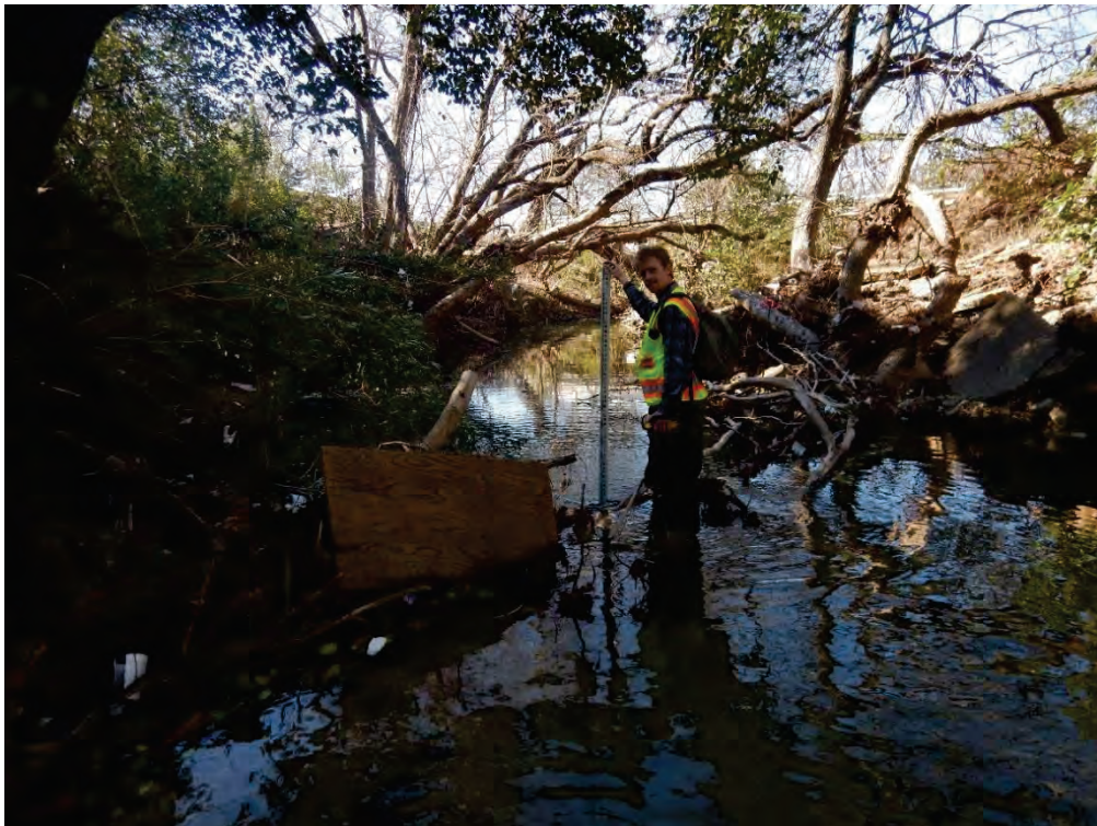
Photo 30. A knickpoint formed by a log jam; there is a 4-foot drop on the downstream side (photo taken looking downstream). There is potential for the knickpoint to propagate upstream when the debris is dislodged.
