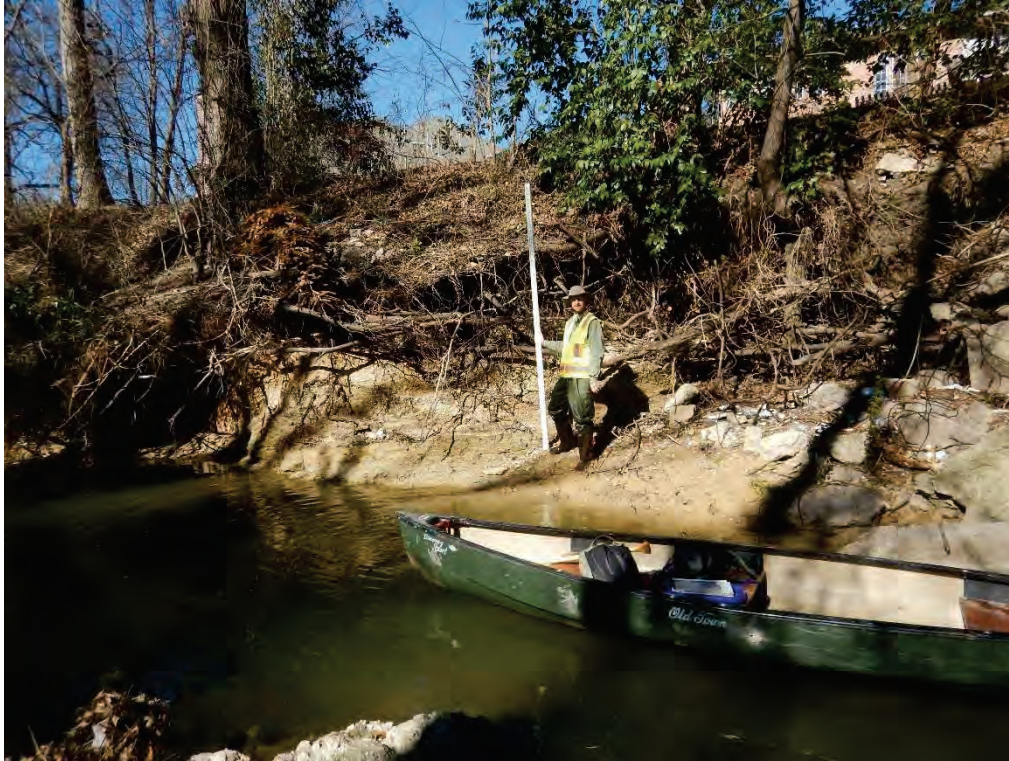
Photo 15. This section of the right bank (15 feet tall) has leaning trees and undercut banks, which indicate high erosion potential. There is private property 10 feet from the top of the bank (photo taken looking at the right bank).
