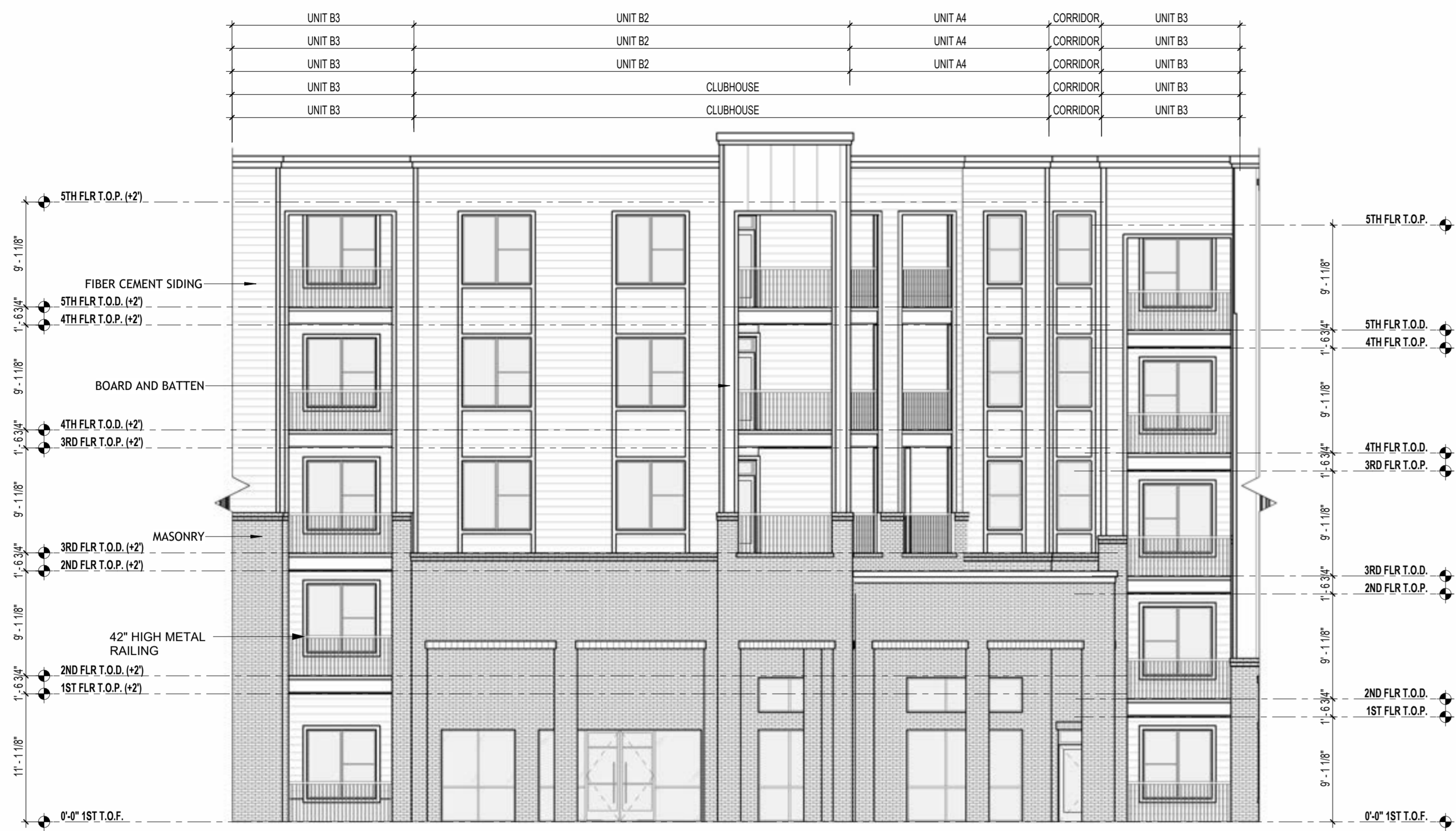
9 BUILDING A - ELEVATION 1/8" = 1'-0"
