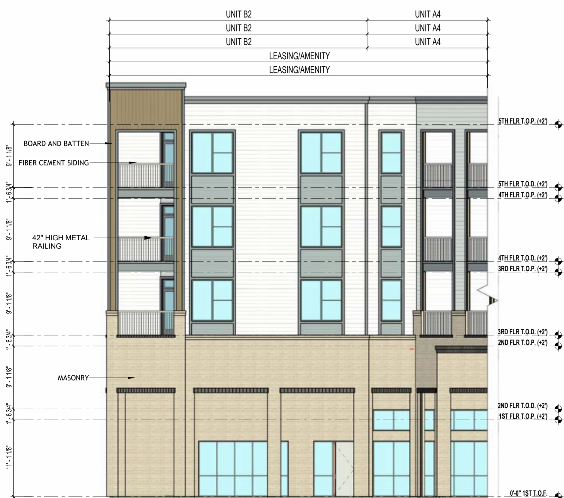
10b BUILDING A - ELEVATION 1/8" = 1'-0"
