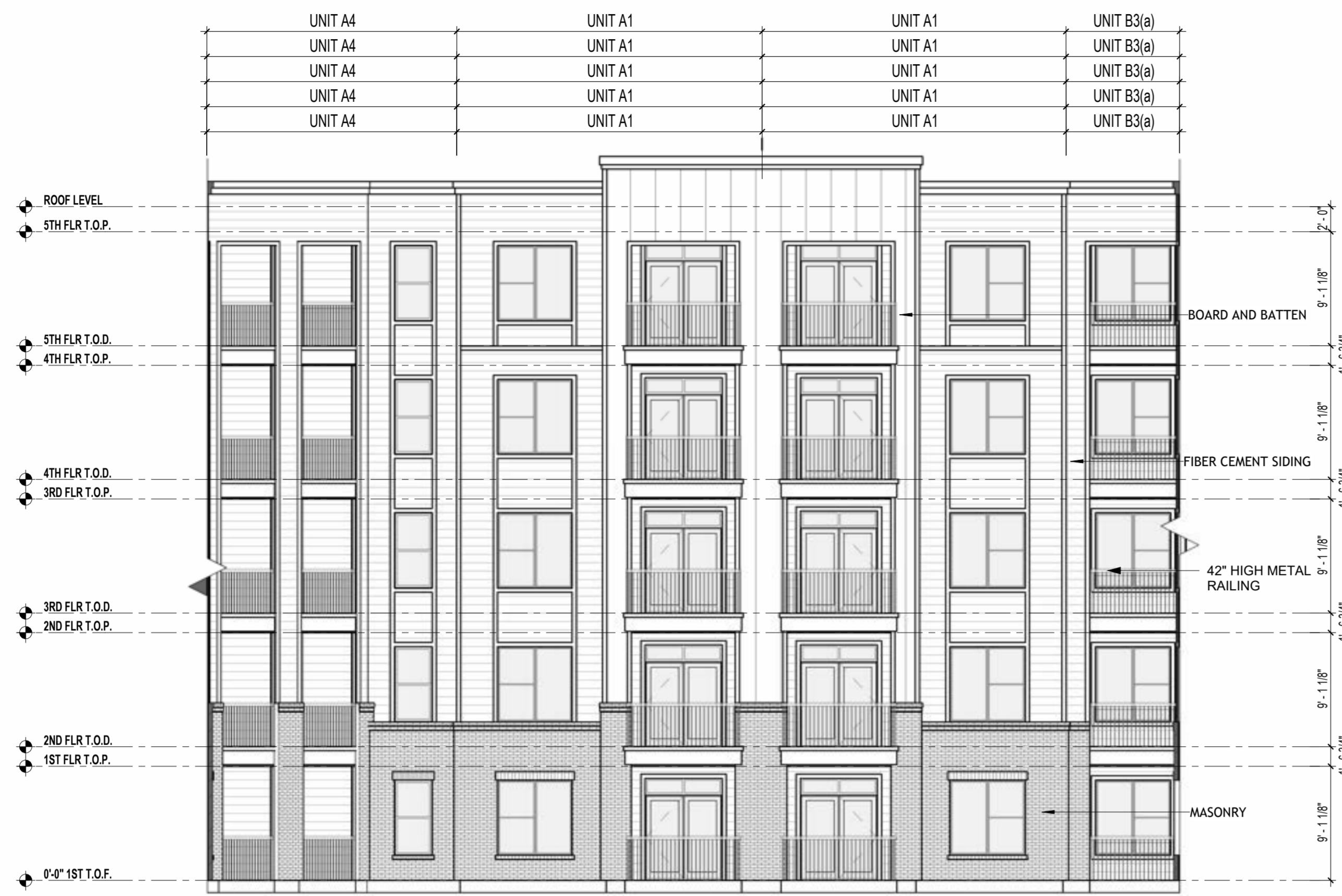
5 BUILDING A - ELEVATION 1/8" = 1'-0"
