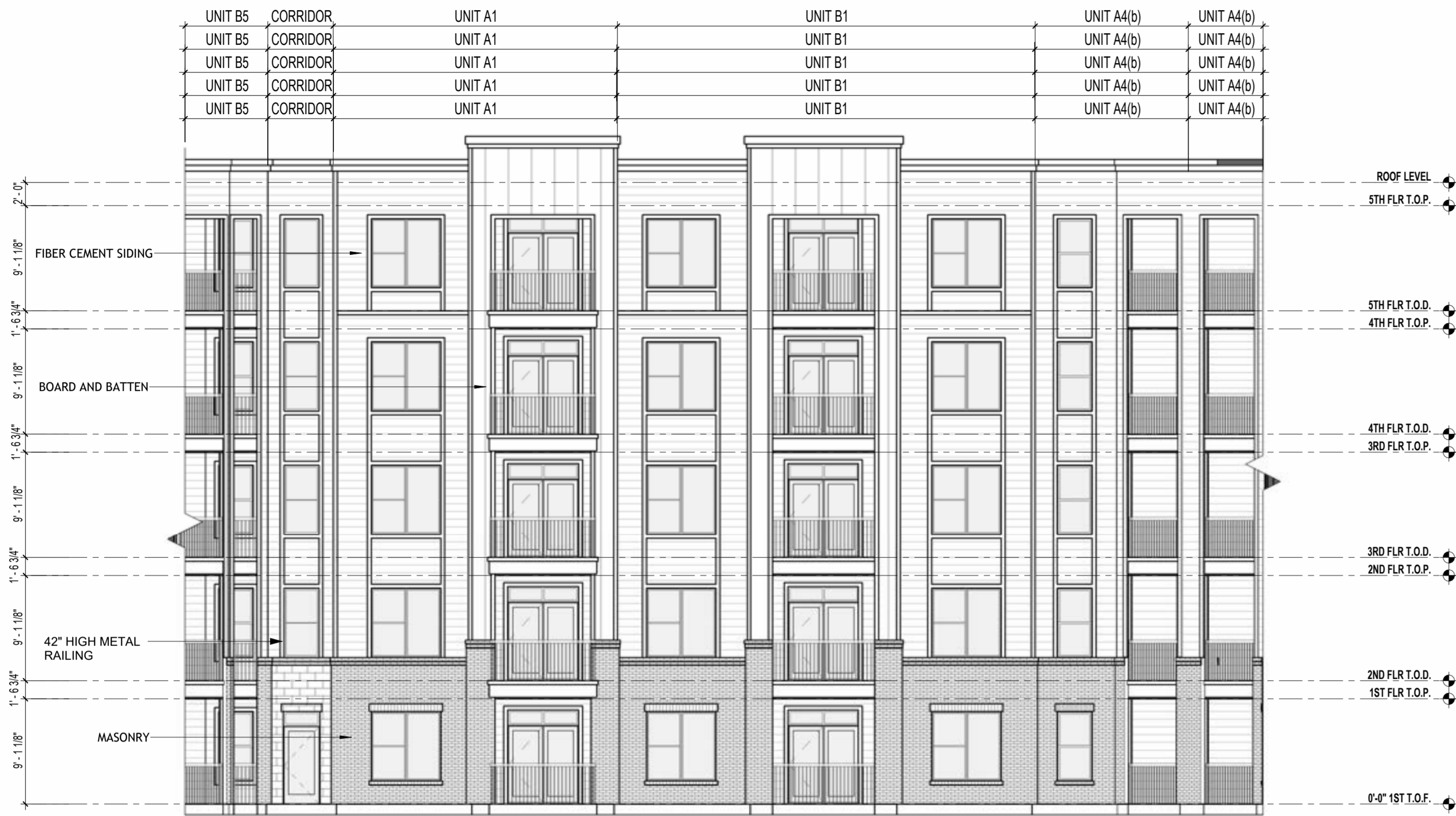
11 BUILDING A - ELEVATION 1/8" = 1'-0"
