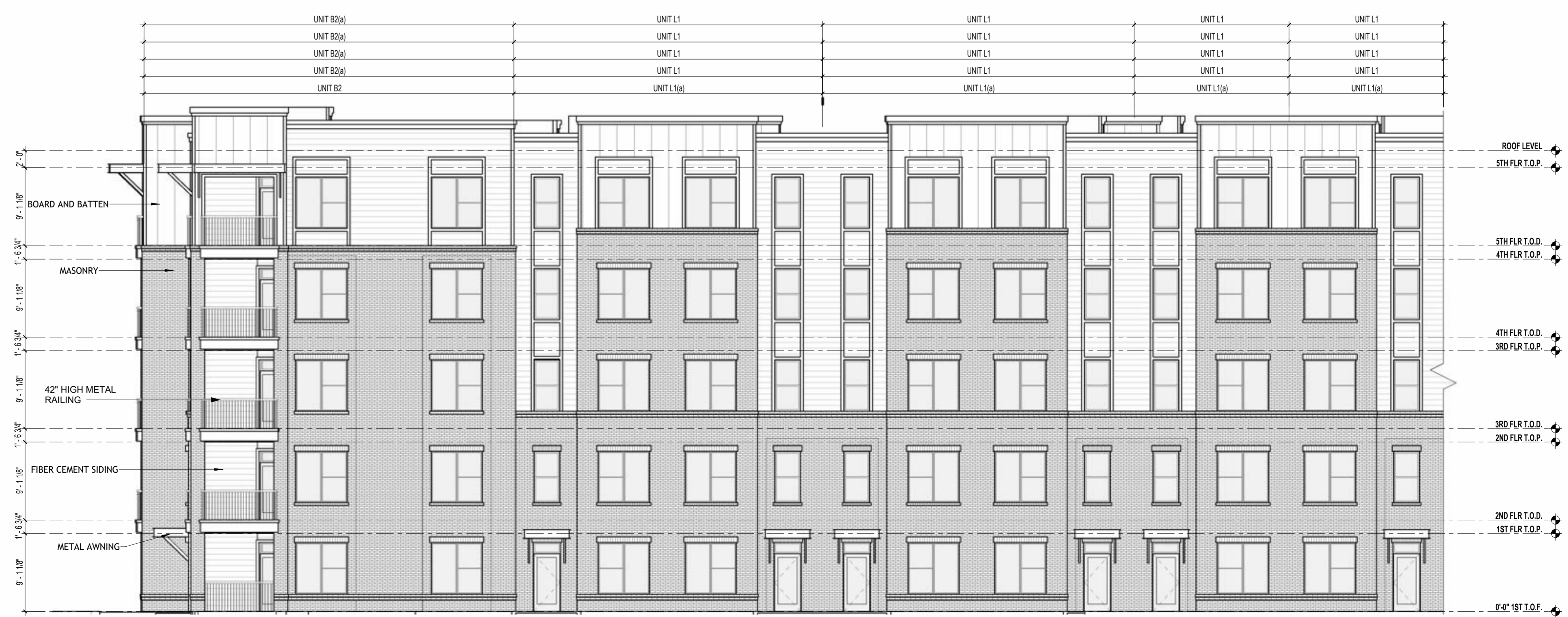
1 BUILDING A - ELEVATION 1/8" = 1'-0"
