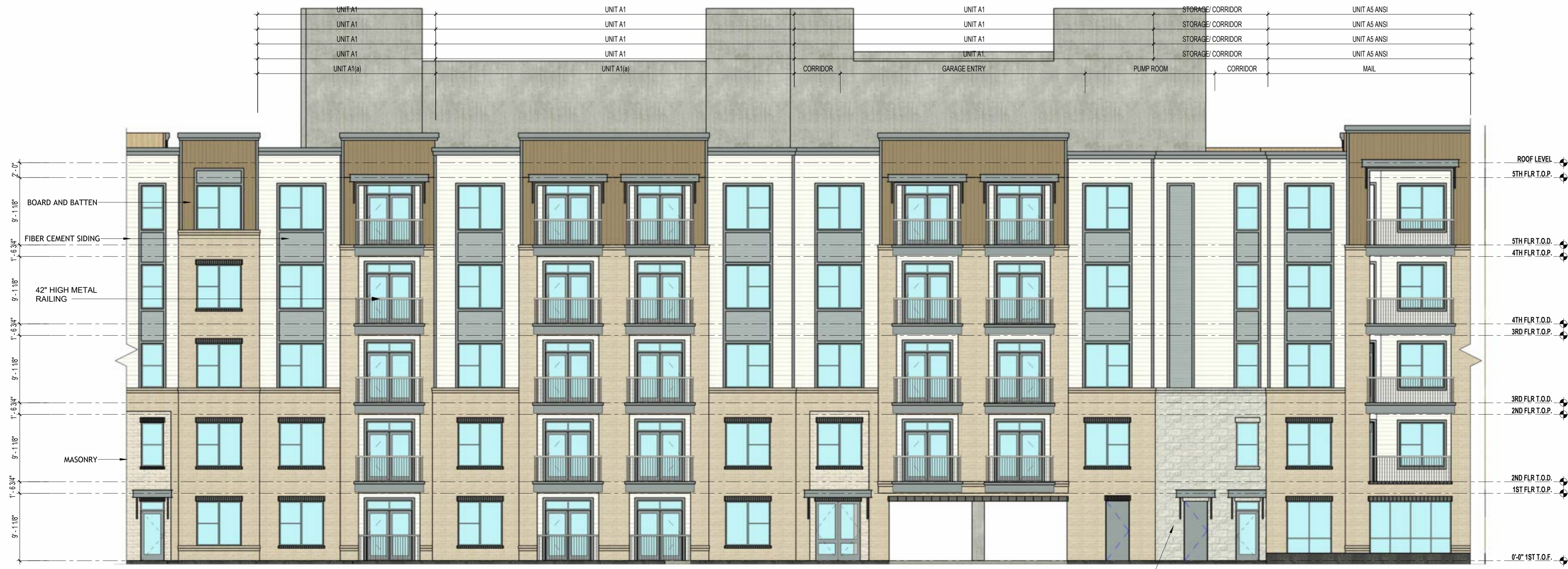
1b BUILDING A - ELEVATION 1/8" = 1'-0"
