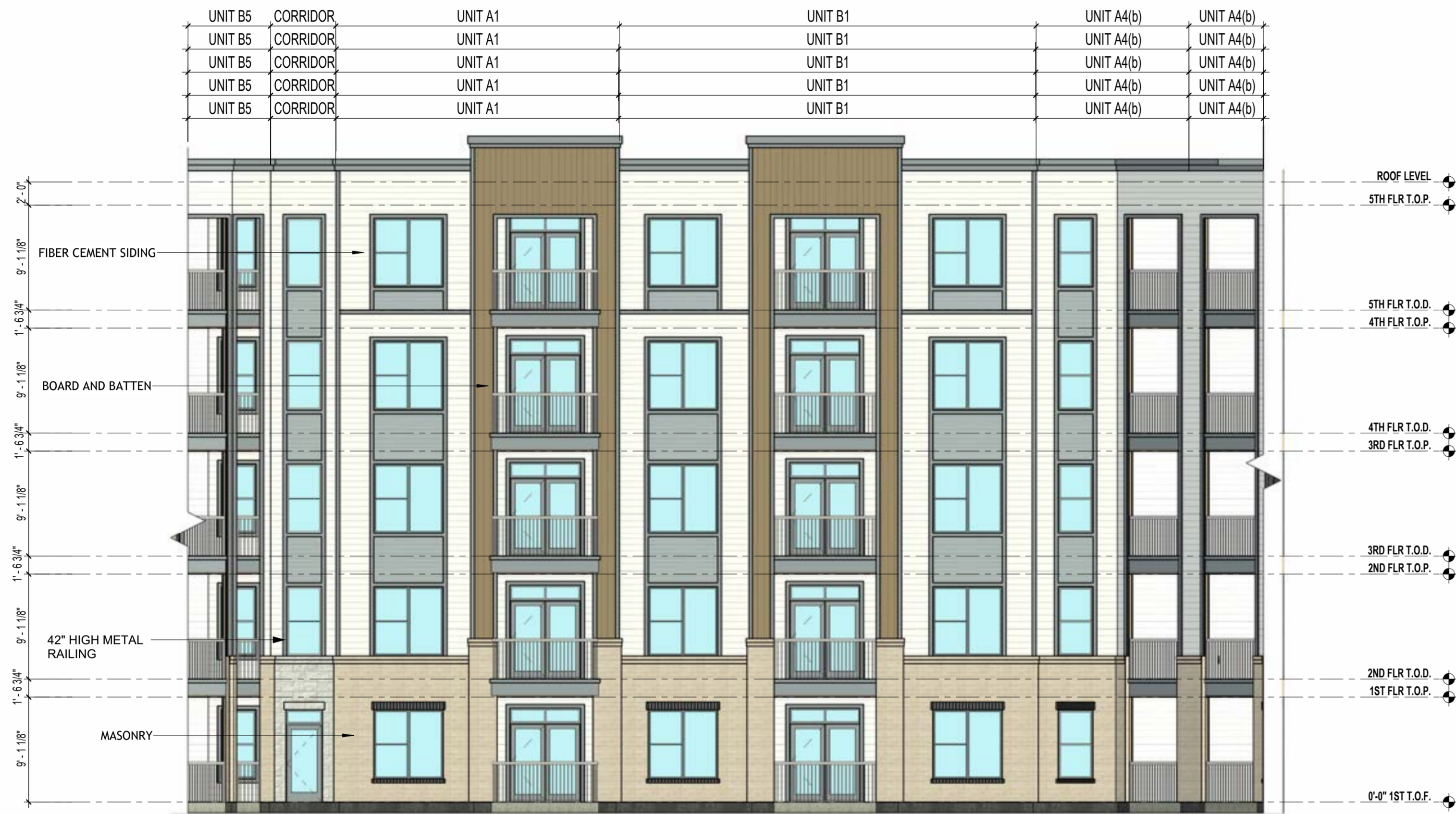
11 BUILDING A - ELEVATION 1/8" = 1'-0"
