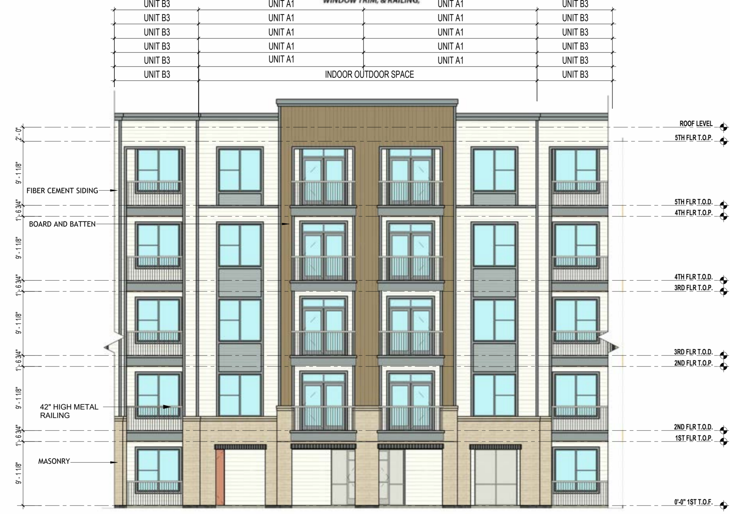
7 BUILDING A - ELEVATION 1/8" = 1'-0"
