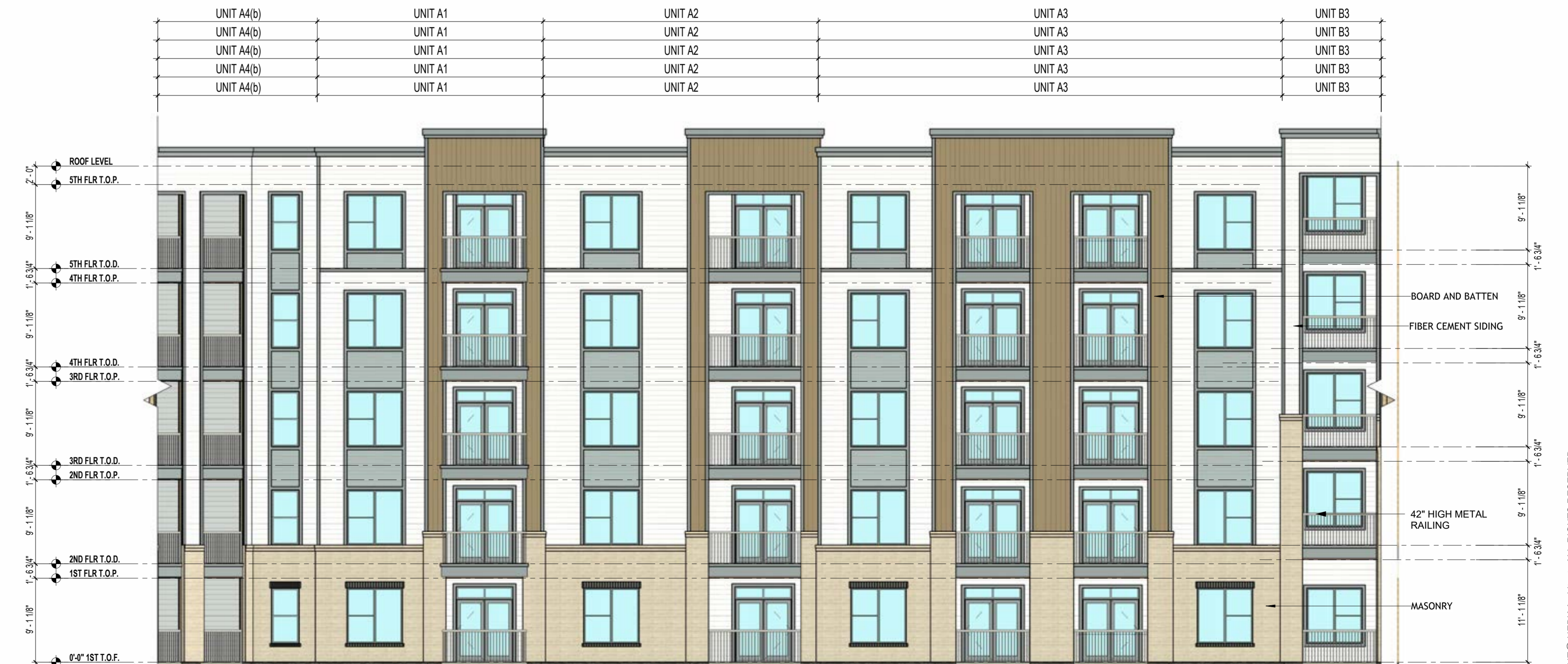
10a BUILDING A - ELEVATION 1/8" = 1'-0"
