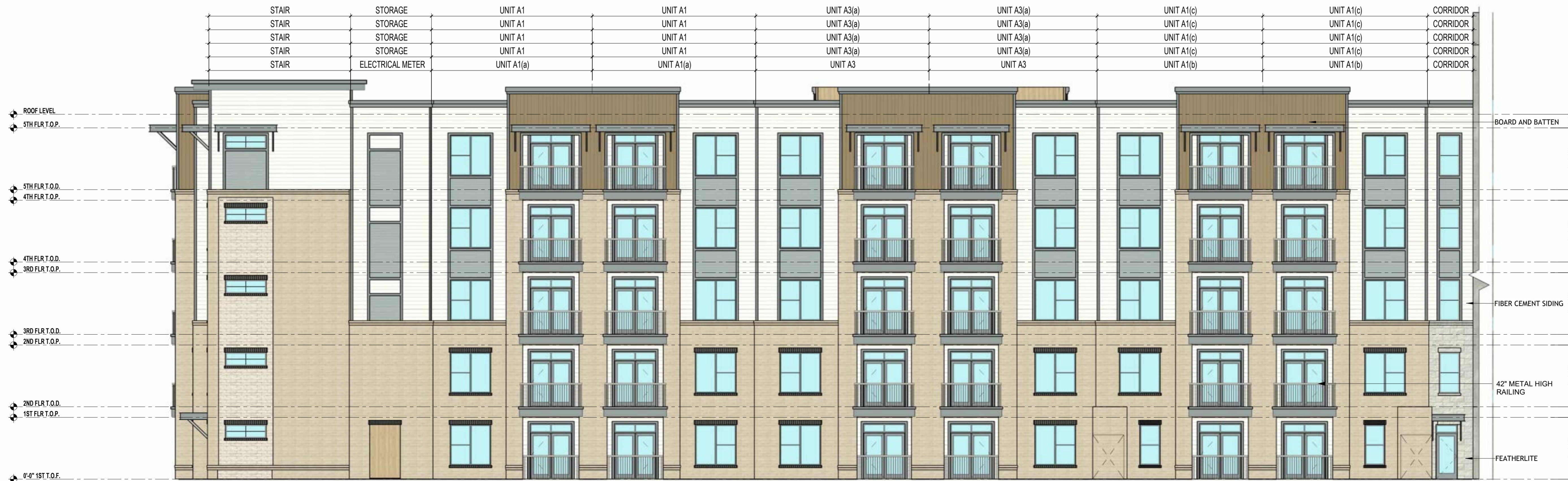
3a BUILDING A - ELEVATION 1/8" = 1'-0"
