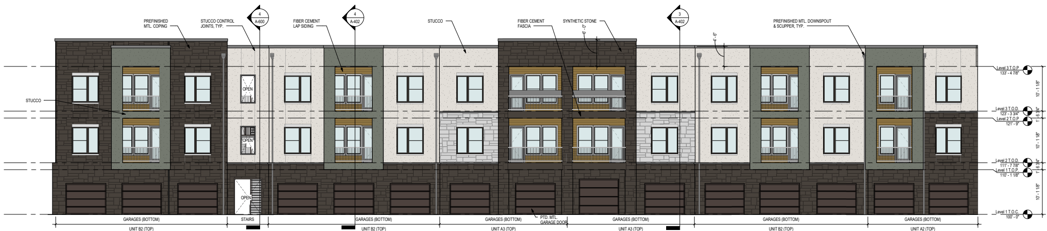
3 Building 2 - South Elevation B 1/8" = 1'-0"
