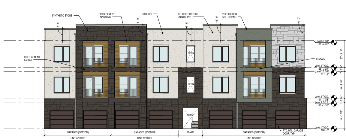
2 Building 2 - West Elevation A 1/8" = 1'-0"
