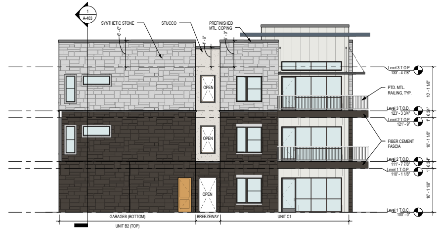
1 Building 2 - South Elevation A 1/8" = 1'-0"
