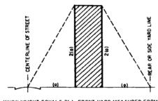
WHEN HEIGHT EQUALS 2(a), FRONT YARD MEASURED FROM STREET CENTERLINE MUST BE MINIMUM OF (a). SIDE AND REAR YARDS WITH OPENINGS FOR LIGHT OR AIR, SHALL BE MINIMUM DIMENSION OF (a) WHEN HEIGHT IS 2(a). IN NO CASE NEED (a) EXCEED FIFTY (50) FEET (SEE 9-502!.)
