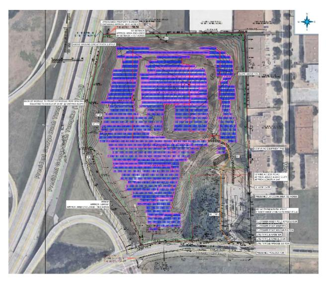
The layouts prepared for the initial system designs consist of what is commonly referred to as a "30% design set." This indicates that the layout is generally about 30% of the way through the engineering and design process that would ordinarily occur to obtain a building and electrical permit, and for an EPC contractor to rely upon during a construction process.
