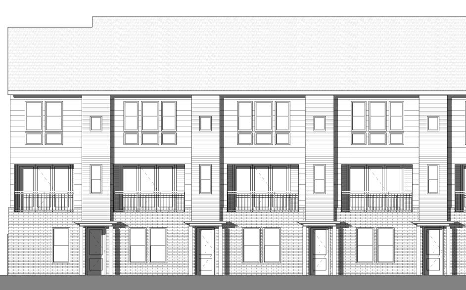
Building 3 - East Elevation Scale: 1/8" = 1'-0"
