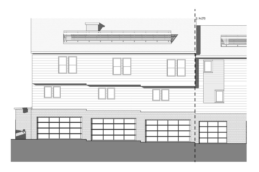
3 Building 8 - East Elevation - Segment B Scale: 1/8" = 1'-0"
