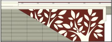
Abutment wall graphic to be installed at Valley View Lane and Valwood Parkway and IH-35E intersections.
